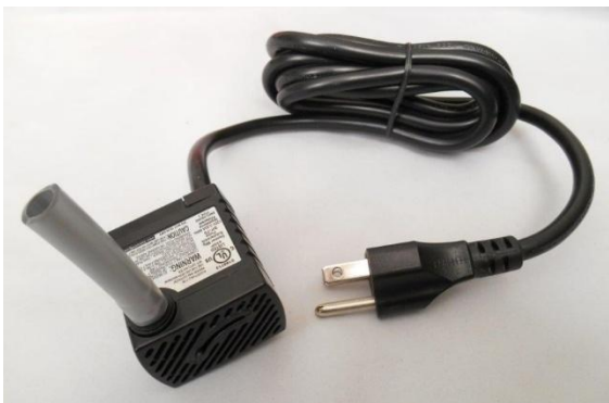
Fig. 3: Assembled Pump with Tygon Tube
