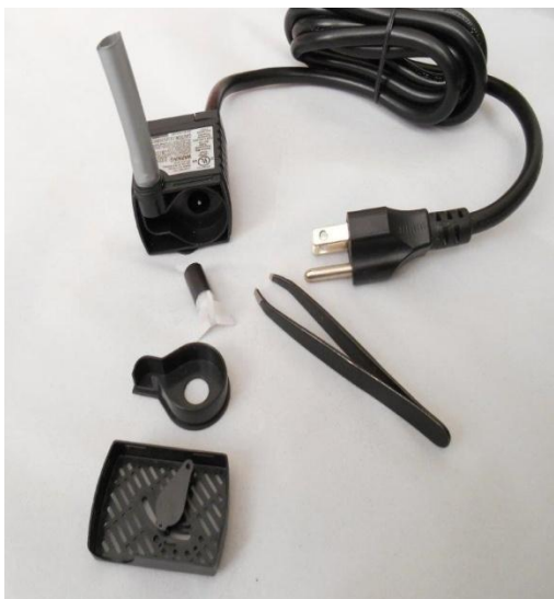
Fig 1: Dissembled Pump with Impeller Removed (and optional tweezers if needed to remove impeller from impeller well)
