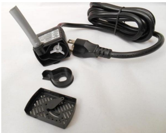
Fig. 2: Dissembled Pump with Front Cover and Impeller Cover removed, Impeller still in Motor/Impeller Well
